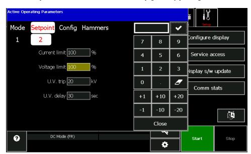
Highlight the U.V.Trip parameter value by touching it. Using the keypad on the right side of the screen press 0 and then press the button to enter the value. Close the window.
